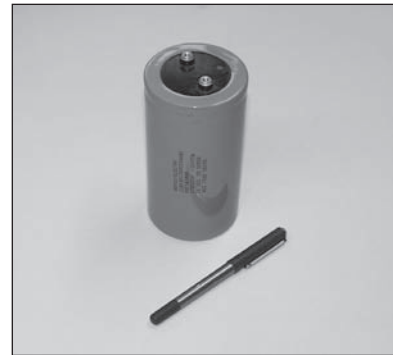
Figure 3.51 (a) Half-wave rectifier circuit with filter capacitor; (b) a-175,000- \mu F, 15-V filter capacitor. Capacitance tolerance is -10 percent, +75 percent.
