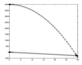
The bottom line shows velocity starting at zero and dropping linearly. The top line shows position starting at 4000 m and dropping parabolically (but remember that this parabola is a function of time, not a ballistic trajectory).
