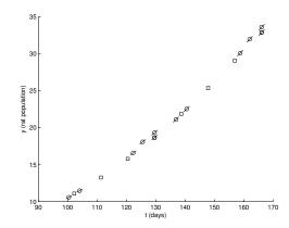
The circles show the points where ode45 called rats. The lines through the circles show the slope (rate of change) calculated at each point. The rectangles show the locations of the estimates  $(T_i, F_i)$ . Notice that ode45 typically evaluates g several times for each estimate. This allows it to improve the estimates, for one thing, but also to detect places where the errors are increasing so it can decrease the time step (or the other way around).
