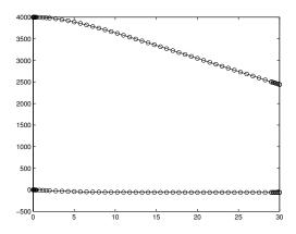
Big difference! With air resistance, velocity increases until the drag acceleration equals g; after that, velocity is a constant, known as "terminal velocity," and position decreases linearly (and much more slowly than it would in a vacuum). To examine the results more closely, we can assign them to variables
